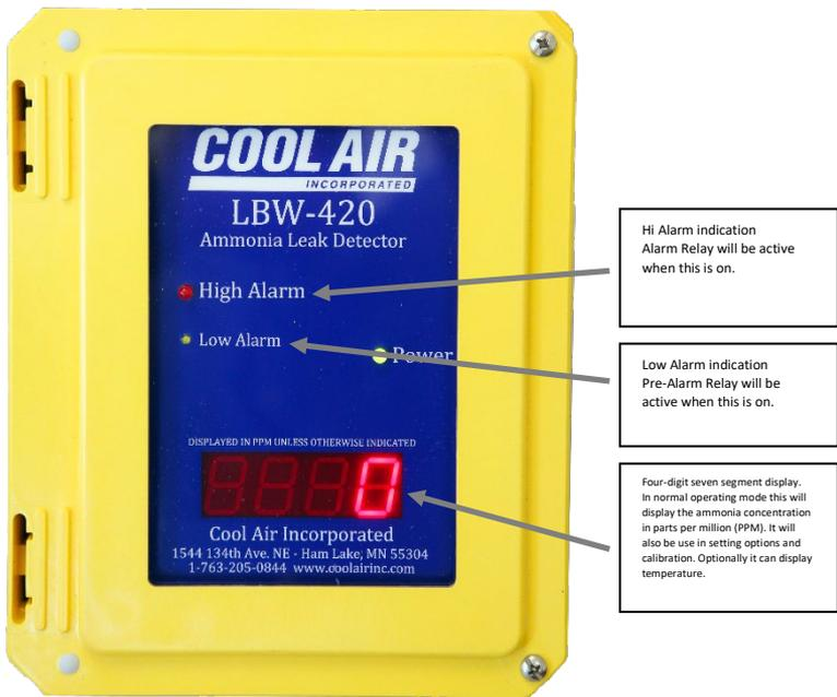
For information on how the display indicates ammonia concentrations, see the sections on ammonia leak indication
