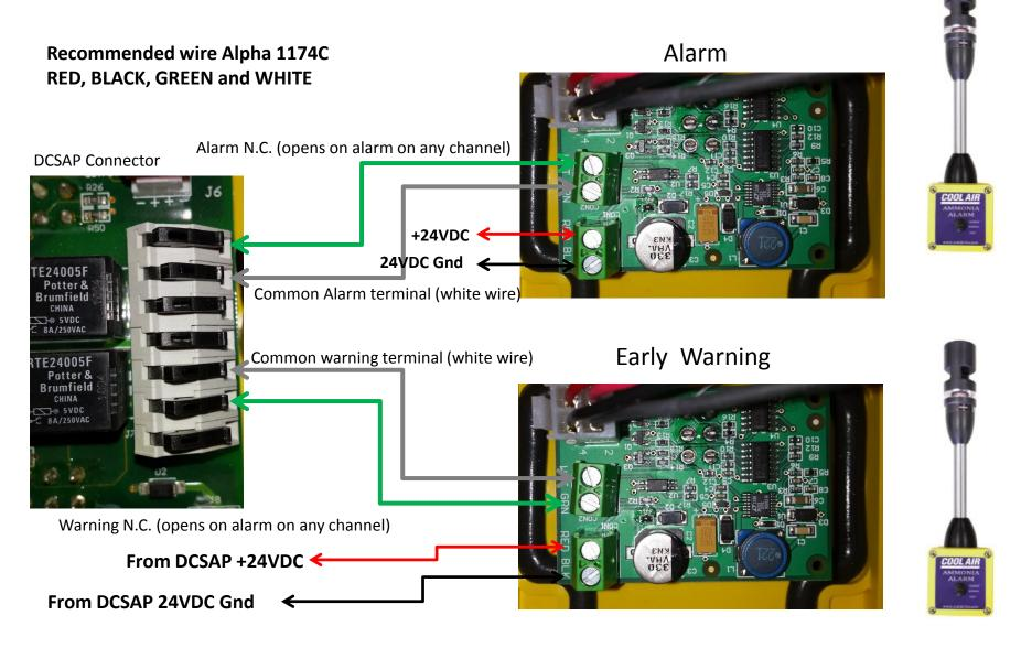
When connecting more than one remote alarm light and horn unit to a set of relay contacts, make sure all white wires are together and all green wires are together. Failure to do so will damage the remote alarm light and horn unit printed circuit assembly.
